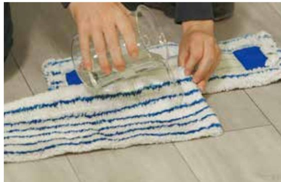
Internal test to simulate wet cleaning. Several mops that are infused with water and a lot of soap (5 times the standard amount), are put on top of a laminate floor with a dampscreen on top to prevent evaporation. This test **determines water leakages between the joints and damages, like swollen edges**.
