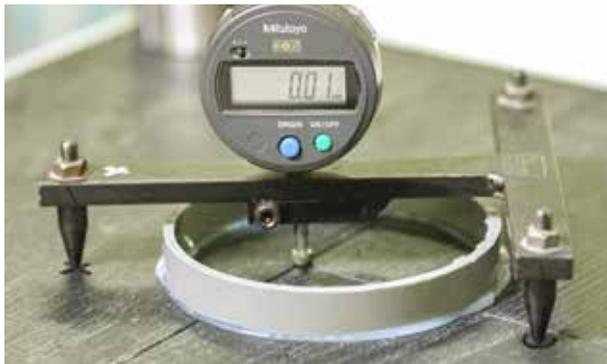
A cylinder with water is placed on the T-joint of a floor. Afterwards the swelling of the material is measured by a measurement device. This test is used to **determine the long-lasting swelling damages** on laminate and other wood-based flooring products. The NALFA test **doesn't measure the watertightness or sealing capacity** of a floor.
