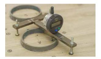
During the NALFA test, a cylinder with water is placed on the T-joint of a floor for 24 hours to determine the long-lasting swelling damages.
