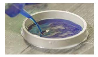
While looking similar to the NAFLA test, the cylinder test **determines water leakages** between the joints during the testing period by adding a white paper or camera underneath the floor to detect any leaks.
