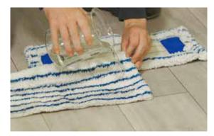
This test simulates wet cleaning: Several mops infused with water and soap are put on the T-joint of a laminate floor. A damp screen is added to prevent evaporation. This test determines water leakages between the joints and damages, like swollen edges.
